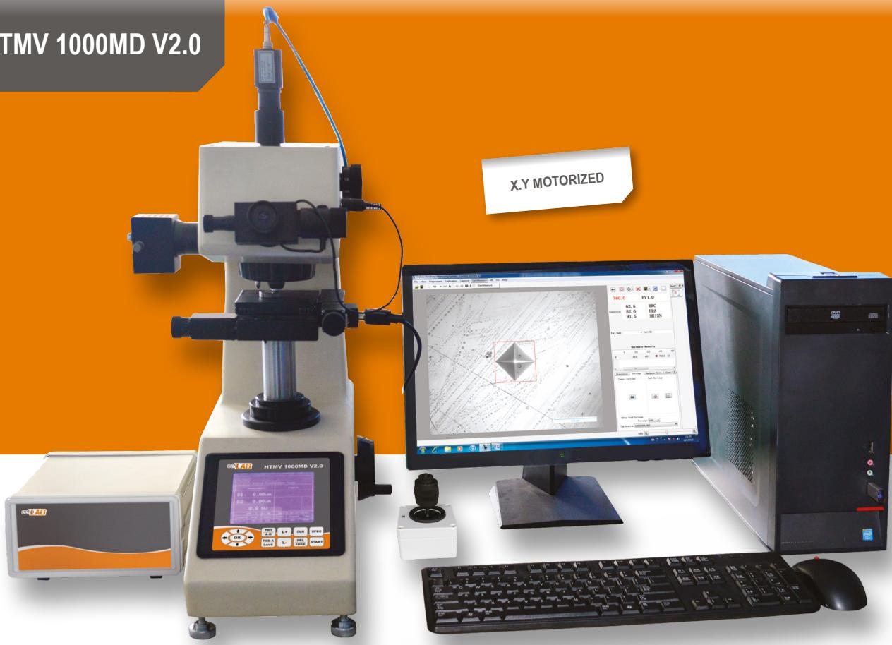
**Automatic Micro-Vickers Hardness Tester**
