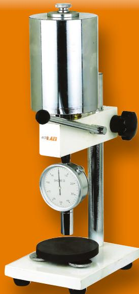
**SHS-A-AC Test stand for Shore Hardness Tester**
