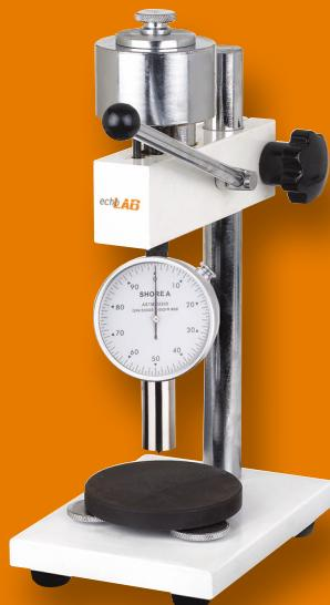
**SHS-A-D Test stand for Shore Hardness Tester**
