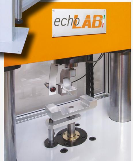
Detections are made using accurate position transducers for acceleration and load.
